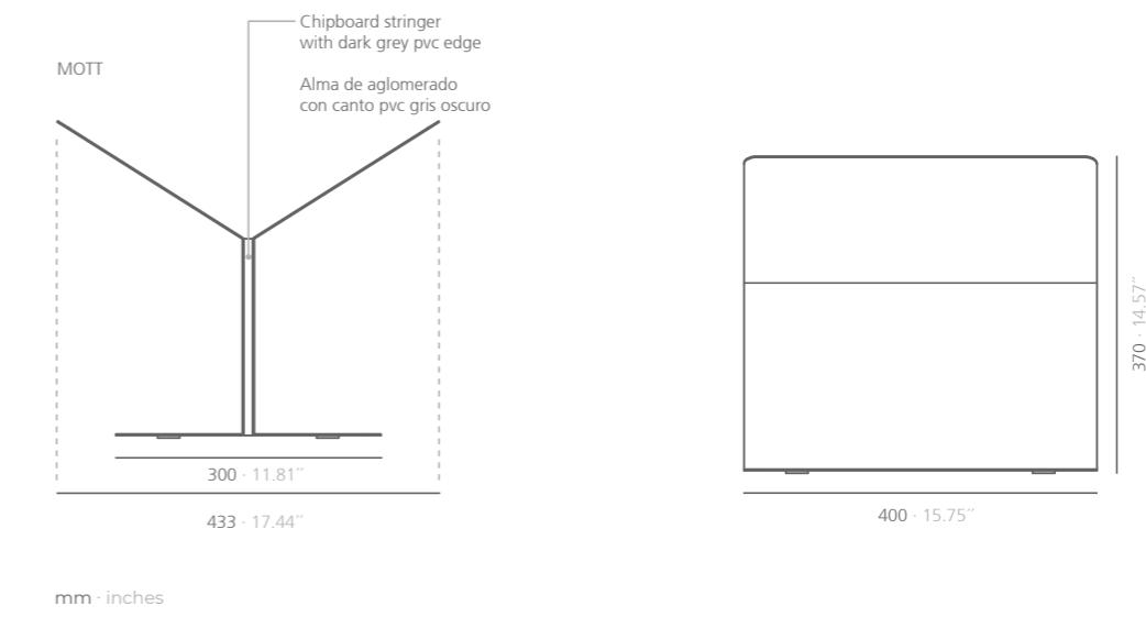
**Magazine rack inspired by architectonic shapes. Made of steel sheet and coated with polyester paint.**
