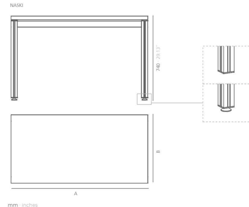
Very stable working tables with a lightweight aluminum structure. Two types of legs available. The tabletops can be soft melamine chipboard or compact HPL.
