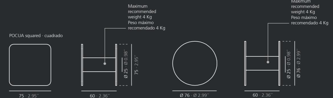
POCUAM hanger with magnetic fixing system for metallic surfaces
