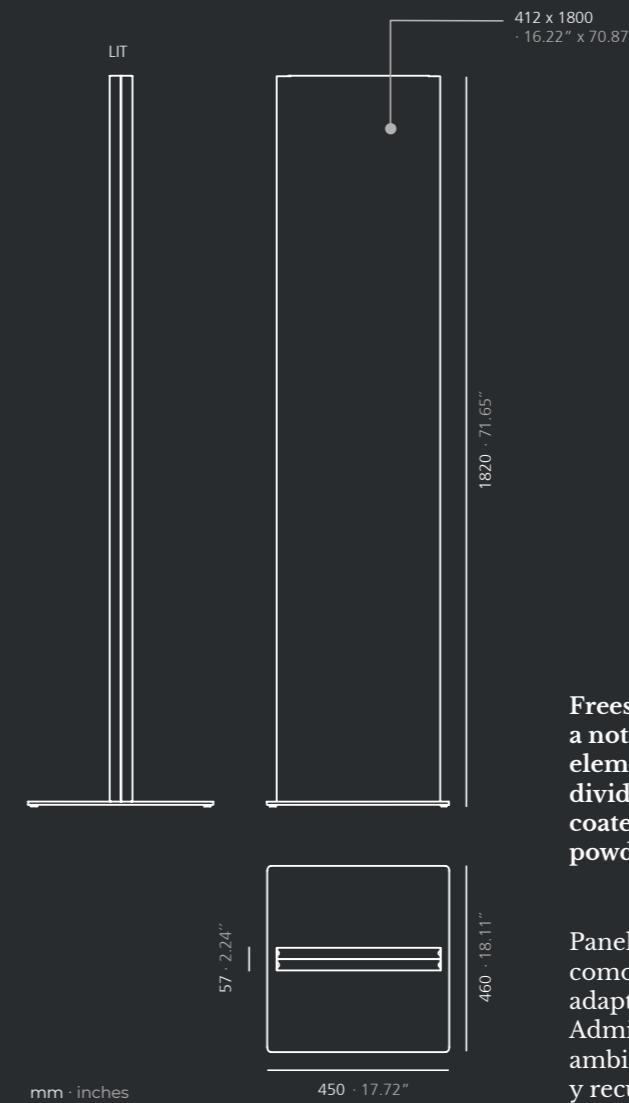
Freestanding vertical panel used as a notice panel by adapting magnetic elements. It also supports the room divider function. Made of steel and coated with oven thermoset powder paint.
