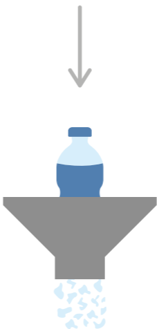
Bottle Flakes and Masterbatch PET bottles are cleaned, shredded into flakes, and combined with masterbatch for colour and performance enhancement.
